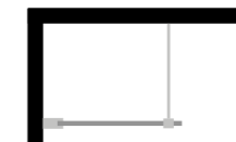
Plan view of flipper panel Left hand corner illustrated Shower screen supplied separately
