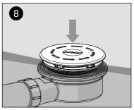
Note: The valve must be pointed towards waste outlet.
