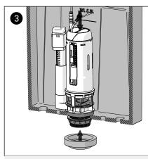
Push down on the valve and rubber seal, and securely tighten the nut. Do not over-tighten. Attach the gasket (not supplied) to the flush valve.
