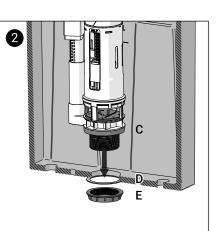
Install the flush valve into the cistern and refit the washer (D), nut (E) from underneath the cistern. Ensure that the rubber seal (C) is inside the cistern.
