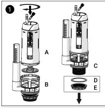
Ensure that the flush valve body (A) is assembled into the housing (B). Remove the nut (E) and washer (D) but ensure that the rubber seal (C) is still attached.
