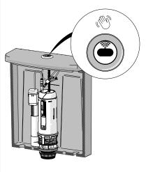
The height of the button's push rod can be adjusted by rotating it. Make sure the bottom end of the rod is touching the manual activator button, and lock it in position by refitting the nut.
