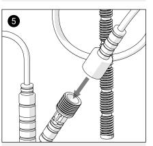
Connect push button to the mechanism.
