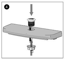
Remove the nut. Fit the push button (G) through the top of the cistern lid. Reattach the nut and secure the push button in place. Do not over-tighten.
