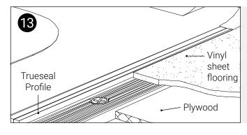
It is important that the Trueseal profile is kept clean and that the protective tape remains intact and is not removed until the flooring is ready for bonding.
