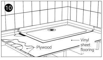
You will need to cover the exposed floor with 4 mm plywood in order to make the floor and Trueseal junction level to apply your vinyl sheet flooring onto.
