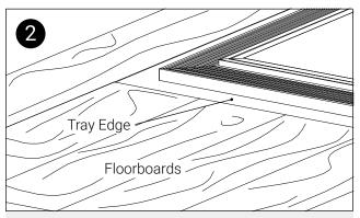
Carefully remove the flooring to the same height as the tray. Do not cut into any plumbing or electrical wiring.
