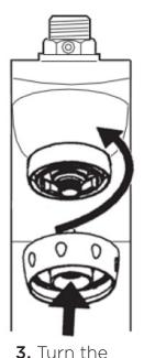
shower head upside down and slot into the locking nut. Unscrew the locking nut and remove.
