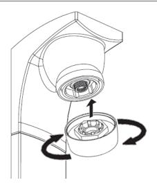
**2.** Invert the spray plate holder and use to unscrew the locking collar.
