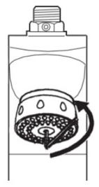
1. Unscrew the shower head using a 4mm hexagonal key.
