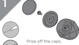
Undo the screws to remove the handles.
