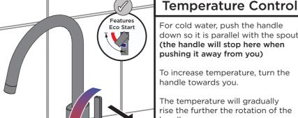
For cold water, push the handle down so it is parallel with the spout (the handle will stop here when
