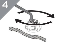
Turn the hexagonal key clockwise to secure the EasvFit Base.
