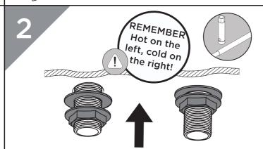
Secure the taps to the basin/bath by using the washer and metal backnut below the basin/bath.
