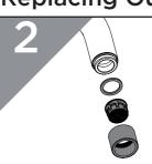
Remove the aerator from housing. Clean and replace as necessary.
