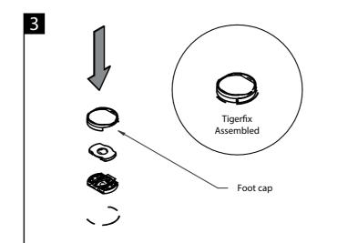
Attach the Tigerfix to the floor within the marked area, leave for 30 minutes to cure.
