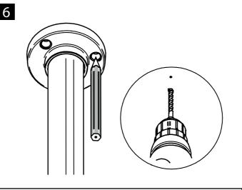
Mark the position of the holes on the ceiling, unlock and lower the inner pole, then drill the positions marked.
