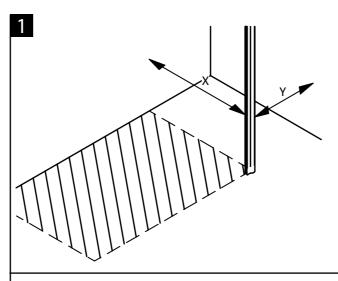
Determine where the first pole of the Aqua- Screen Clear Walk Through is going to be.
