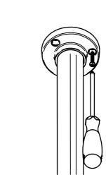
Raise the inner pole, lock in position and screw the ceiling bracket in place. For the optional threshold strips installation go to pages 3 -5 (main installation guide).
