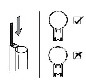
Slide the flipper seals down into both telescopic poles and cut off any excess. Note the orientation of the soft flippers.
