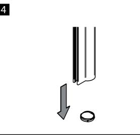
Position the outer pole on top of the Tigerfix as shown.
