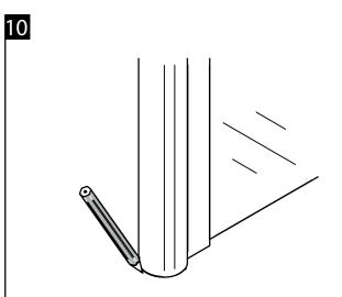
Mark location of the other pole as shown. Then repeat stages 3-7 to complete the installation of Aqua Screen Clear Walk Through.
