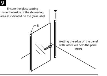
Attach the other telescopic pole (B) to the panel, then place the glass panel (correct way around) into the floor to ceiling pole as shown.
