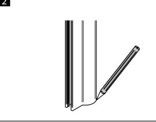
Mark location of the floor to ceiling pole as shown.
