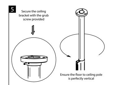
Fit the ceiling bracket to the inner pole. Then extend the pole to required height and rotate it until it locks into
