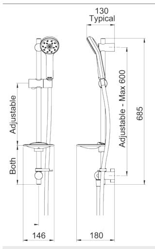
CONSTRUCTION: Stainless steel/ABS SUPPLY: Suitable For Low Pressure Systems INLET CONNECTIONS: ½" BSP WORKING PRESSURES: 0.3 - 5.0 bar CARTRIDGE/VALVE TYPE:N/A
