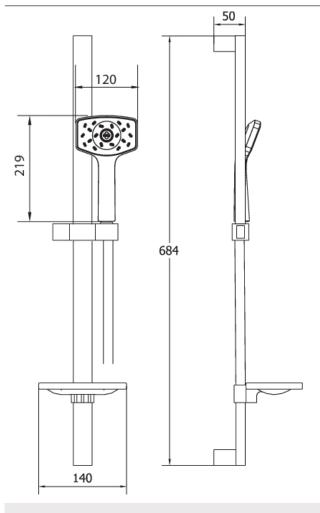
**CONSTRUCTION**: Stainless steel/ABS **SUPPLY**: Suitable For Low Pressure Systems
