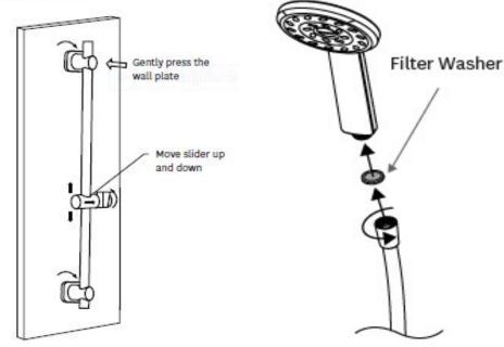
Use a 6mm drill bit to drill a hole in the wall at the desired height, drill a second hole vertically lower at a recommended height of 550mm. In certain
