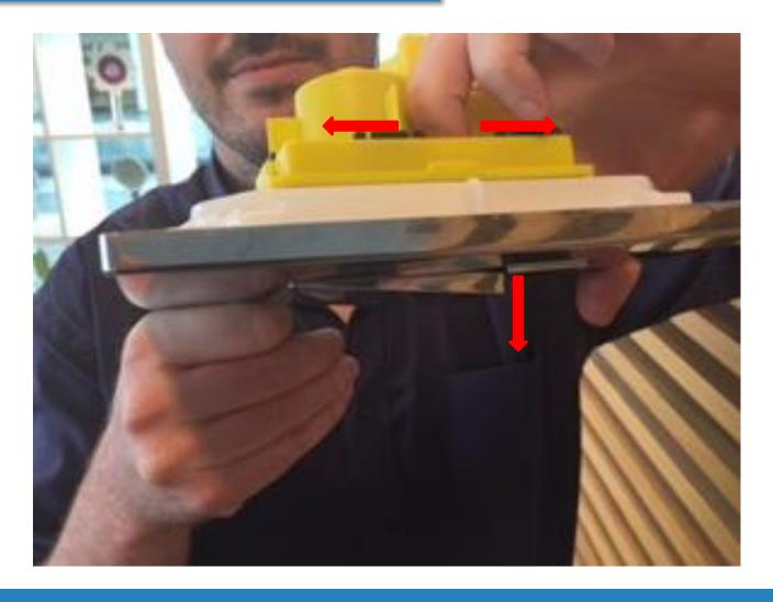
Depending on how you are hold the plate, either pull or push the black legs to partially release the large button (see above pic)
