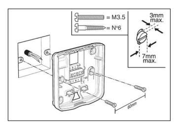
CAUTION – isolate power supply and make safe before wiring the unit to prevent electric shock and equipment damage. Installation should be carried out by a qualified Electrician or competent Heating Engineer.
