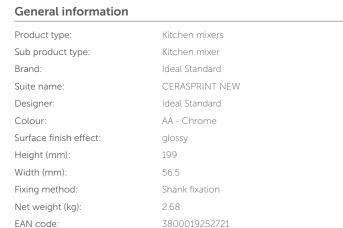
Suitable for high pressure balanced supplies. Inlets with flexible hoses with connections screwed 3/8" BSP female. Unregulated flow rate 7 litres per minute at 1 bar and 12 litres per minute at 3 bar.
