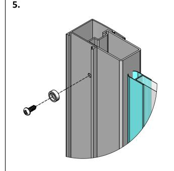
FIX YOUR SCREEN IN PLACE, USE A 3mm DRILL BIT AND DRILL THROUGH THE HOLES IN THE WALL PROFILE.
