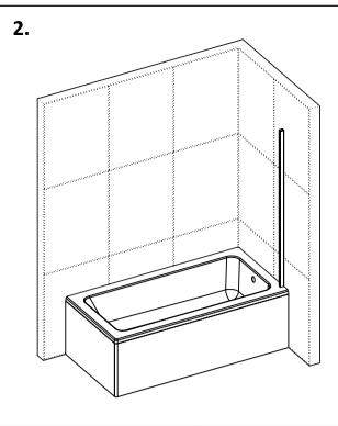
REPLACE WALL PROFILE WHERE MARKED AND MARK THROUGH THE FIXING HOLES WITH A PENCIL.
