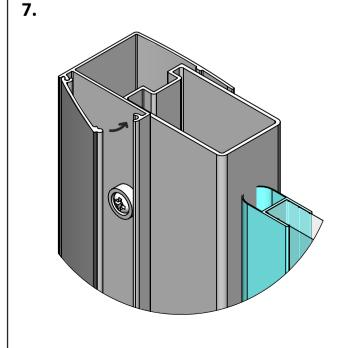
TO FIT THE COVER PROFILE (ITEM 3) HOOK AT THE REAR FIRST THEN SNAP INTO PLACE.
