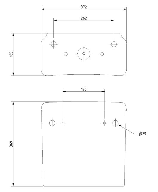
Cistern fitting pack for close coupled rimless pan
