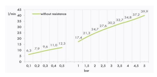
Procedure:Pressure:Cold:Hot:To 38 deg C:Flow Determination3,0 Bar18,9 l/min19 l/min26 l/min
