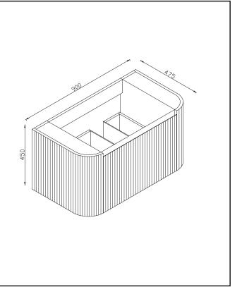
Dimensions (Measurements in mm)
