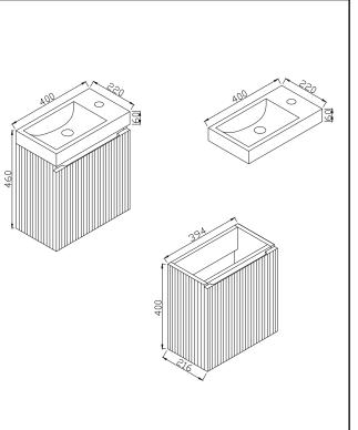
Dimensions (Measurements in mm)
