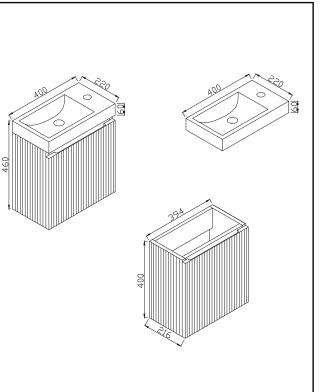
Dimensions (Measurements in mm)
