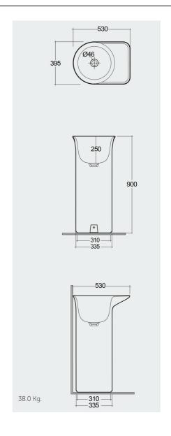
Dimensions: All dimensions in mm. Tolerance of vitreous china & fireclay items:  $\pm$  5% for below 200mm and  $\pm$  3% for above 200mm; for all other items tolerance  $\pm$  1%. Note: Due to a continuing development program to improve design and performance, the manufacturer reserves all rights to vary specifications without prior information. Please note accessories are for photographic use only.
