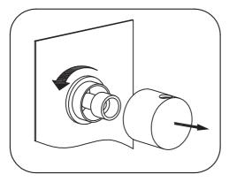
In the event that you should need to remove the flow control valve, first turn off water supply.
