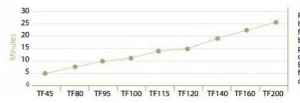
Predicted heat up times for cylinder based on test procedures defined in BS1566:2002 for type P cylinders.
