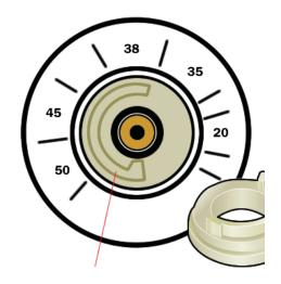
With the Chrome dial removed you will see a plastic ring covering with the Thermostat underneath.
