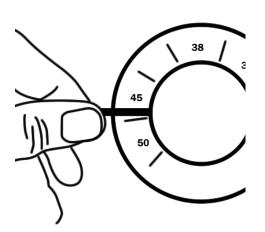
Using a 2.5mm Alan key, insert this into the hole where the chrome cap was fitted and loosen the grub screw about 1 turn to loosen.
