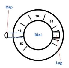
From inside the shower, on the lower of the three dials, remove the chrome coloured plastic cap that is fitted on the opposite side to the chrome lug.
