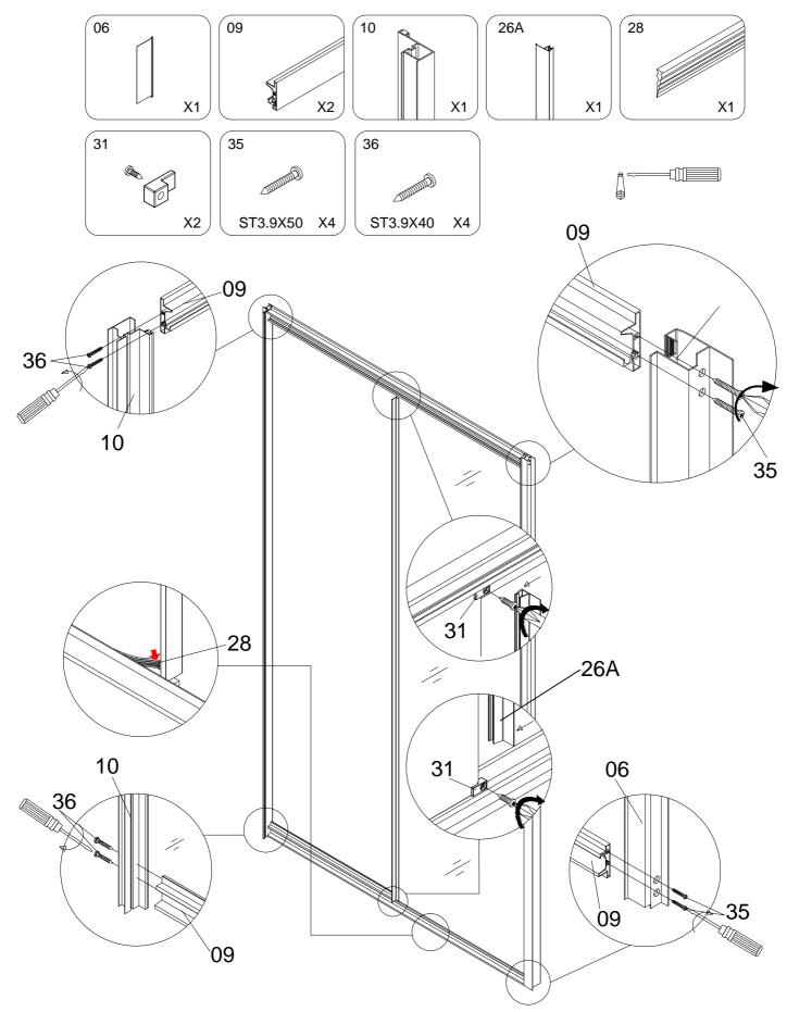
Locate the two silver coloured upright frame sections and the top and bottom frame rail sections. You will need the ST3.8  $\times$  50mm on the left side and the 40mm on the right to join these sections together.
